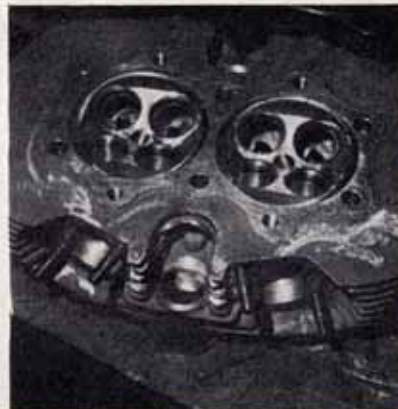
Right valve area can be arranged in the compact design of the Rickman-Weslake head, allowing high c.r. and well-placed plug
