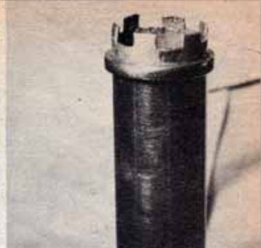
About 1/8 in. may have to be ground off the top of the exhaust pushrod tube and an extension spacer is fitted below seal
