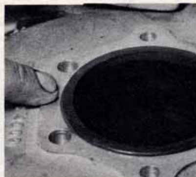
The barrels are spigoted, make sure that the heads seat properly before starting to tighten them down
