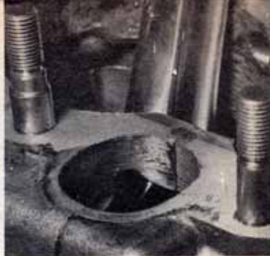
As the cylinder head is wider than the Triumph one, the tappet guide wells have to be opened up to suit splayed tubes
