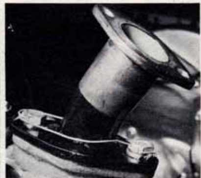
Intake stubs were not supplied with this kit and were made up. They may be splayed or parallel, with length 2.25 in.
