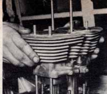
The alloy barrels are fitted on to long studs which run all the way up into the head. Larger bore gives capacity of 683 cc
