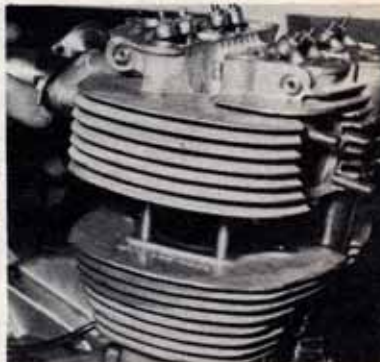
Fitting the heads. Note that the tappet position relative to the cam has been changed, re-timing is explained below
