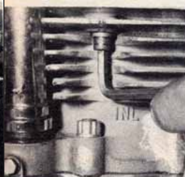
The head is secured by four studs running through block, two studs from block and these Allen screws beside inlet pushrods
