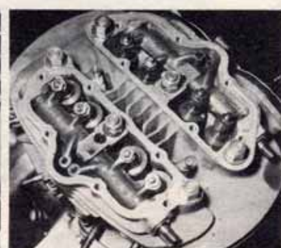
One rocker operates each set of twin valves, the valve clearances, set cold are .011 in. inlet and .013 in. exhaust
